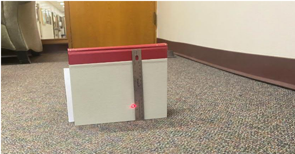
Laser dot shows the vertical settlement of the floor slab.
